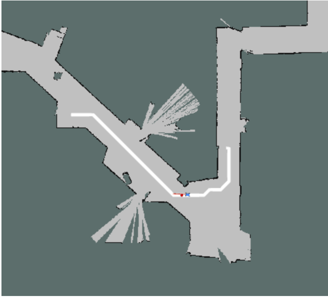
Fig. 12: The racecar following the trajectory in simulation. The red dot indicates the closest point, from which we calculate the error of the pure pursuit algorithm in following the trajectory
