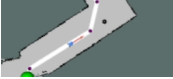
Fig. 7: Pure pursuit based on intersection point. The car follows the closest intersection point through calculations based off the slope.
