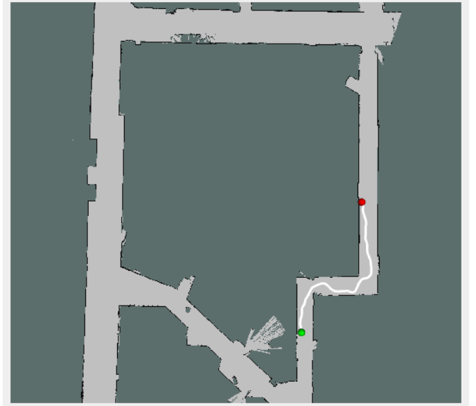
Fig. 5: A path generated by RRT* with dynamics. The initial pose of the robot (the green node) was facing towards the top of the image. The robot is able to preemptively turn to make the tight corner.
