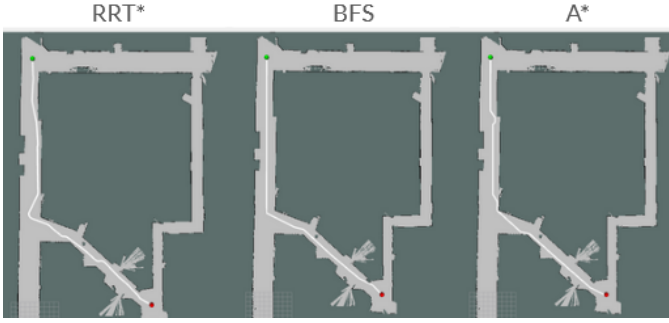
Fig. 10: Our three algorithms all finding a path on the same initial conditions. RRT* and A* seem to cut some of the corners too closely. Because RRT* incorporates the dynamics, these trajectories should be possible, but they are still worth noting.
