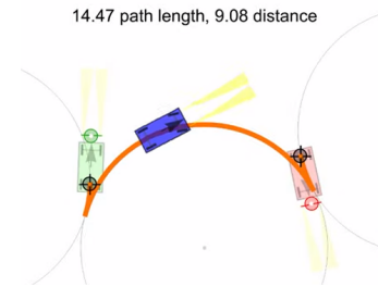
Fig. 9: A Reeds-Shepp curve between two car poses. The green pose is the initial pose, blue is an intermediate pose, and red is the final pose. The initial and final poses point in opposite directions and reverse on the first and third segment.
